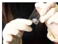
Mother material YCrB4 for hydrogen boride synthesis
